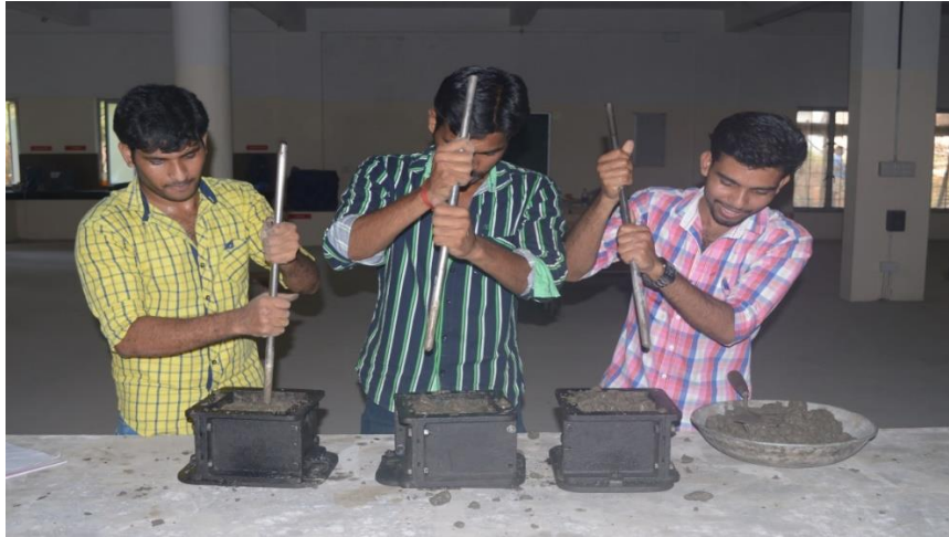
Fig 6.4.2: Removal of air voids
